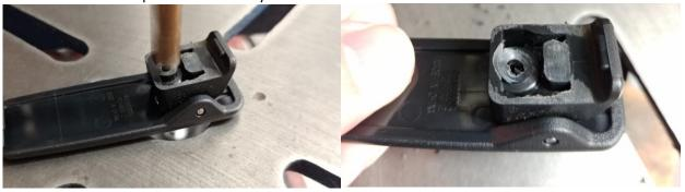
Now, back in a vice I used a small chisel to knock a small notch in the middle of the flat rectangular part to fit the upper portion of the "key notch" in the back of the radio.
