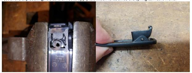
Next, use a 5/16" drill to put roughly 1/16" deep recess in the area where the screw hole is to match the circular portion of the "key notch" on the radio
